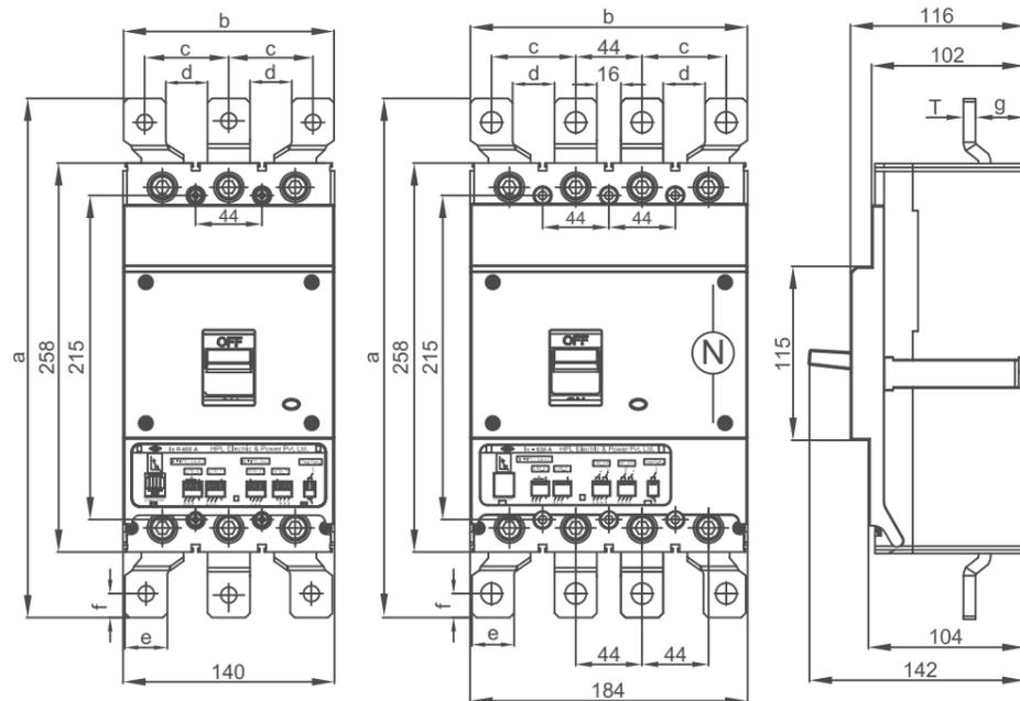
Note: All dimensions are in mm with ± 5% Tolerance.
